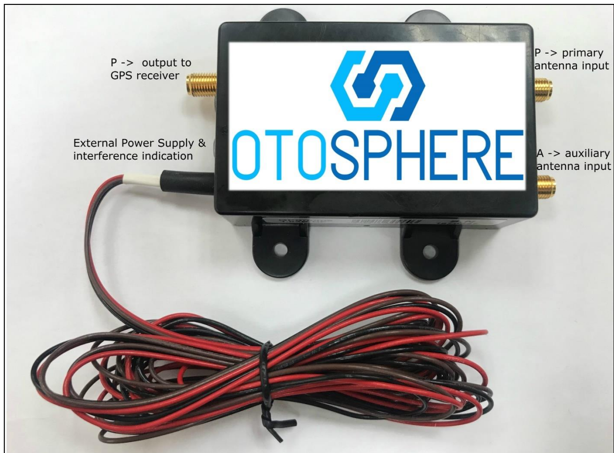
Figure 1 - OtoSphere v1.0-EPS - General Overview
