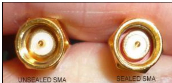
Figure 3 - Unsealed vs Sealed SMA Connectors
